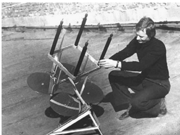
Fig. 8.18. Concentrator PV installation with four parabolic mirrors and AlGaAs/GaAs cells mounted on the heat pipes, 1981 [117]. In photo: Rumyantsev
