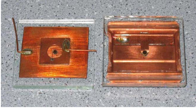
Fig. 8.25. Small-size ( 2 \times 2 \text{ mm}^2 ) cells mounted by soldering to: flat copper plate ( left ) and trough-shaped copper plate ( right ). In the latter case, a heat-sinking trough with a string of cells can be placed behind a glass sheet
