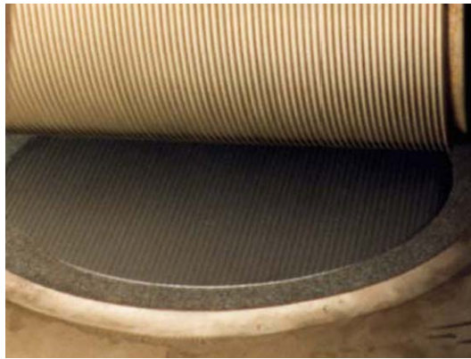
Fig. 6.5. High-throughput grinding tool for surface grooving of OECO solar cells. A 10 \times 10 \text{ cm}^2 wafer can be processed in a few seconds
