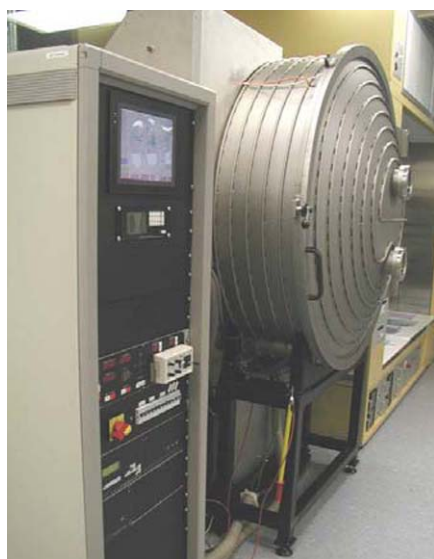
Fig. 6.8. Prototype of high-capacity oblique evaporation equipment for the metallization of OECS solar cells. Large wafer cassettes are arranged on a cylinder revolving around the evaporation source
