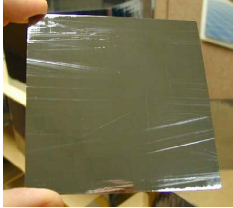
Fig. 5.7. EFG wafer produced by using a laser to cut the octagon tubes with a laser
