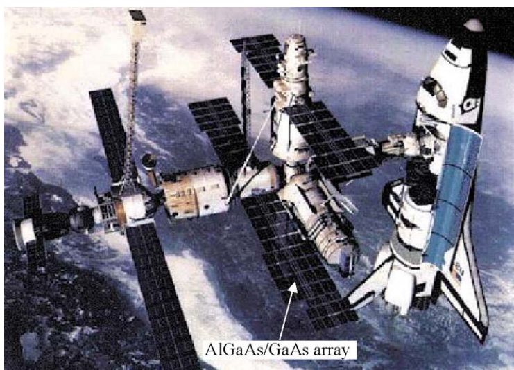
Fig. 8.1. Command module of MIR Space Station was launched into orbit on March 13, 1986, with a PV array based on AlGaAs/GaAs solar cells developed by the Ioffe Institute and fabricated in NPO Kvant. The array operated during the entire 15-year space station mission
