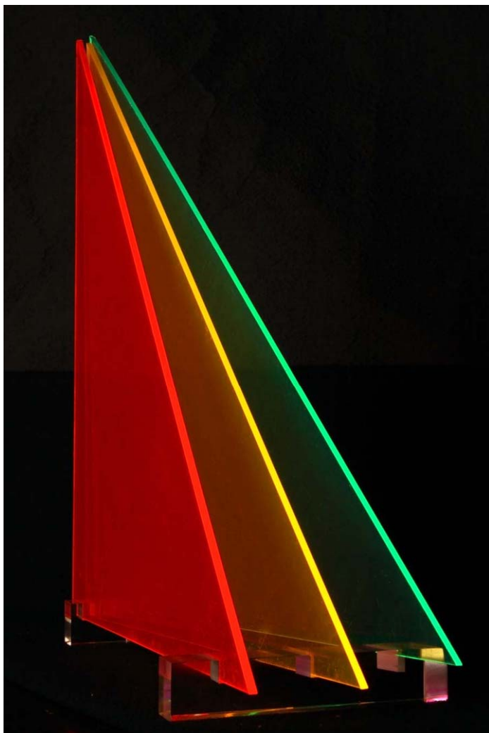
Fig. 10.15. Three PMMA plates doped with different color dyes. These plates are about 25 years old but not degraded, they were however mostly stored in the dark. Although the light output looks very spectacular only part of the light arriving at the edges is emitted because a big part is reflected back by total internal reflection
