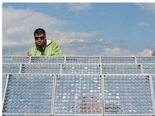
Fig. 8.22. Array of the full-size concentrator modules with small aperture area Fresnel lenses [130]
