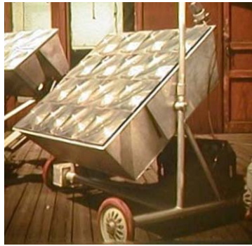
Fig. 8.20. Solar PV installation with 16 Fresnel lenses ( 25 \times 25 \text{ cm}^2 each) and AlGaAs/GaAs cells, 1986 [119]
